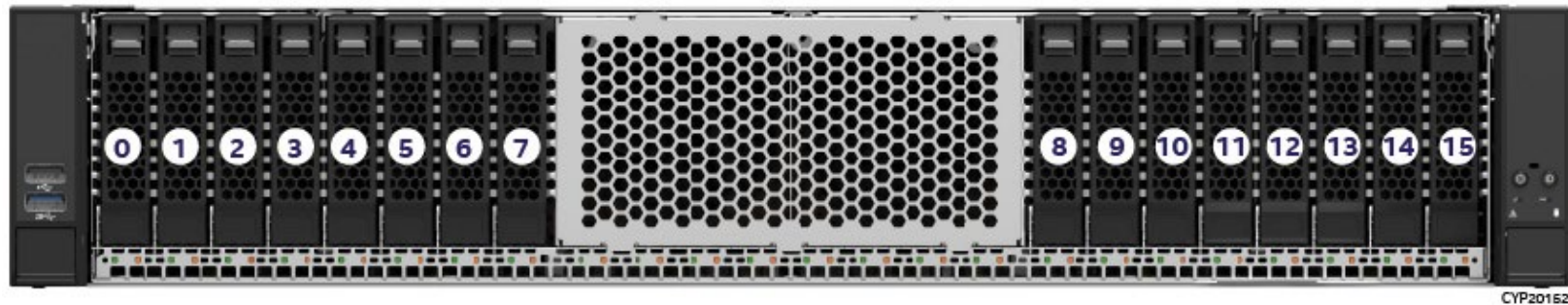
Figure 24. 2U 16 x 2.5" Front Drive Bay Configuration
