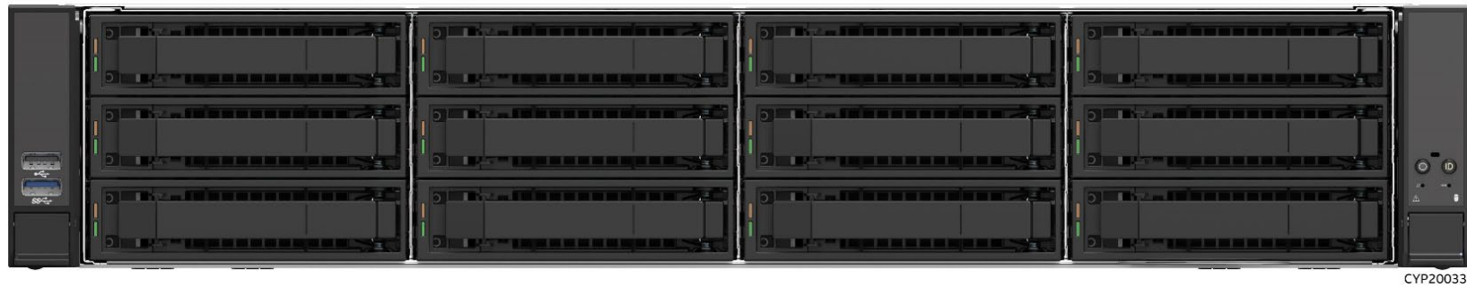
Figure 12. 2U 12 x 3.5" Front Drive Bay Configuration – iPC M50FCP2UR312
