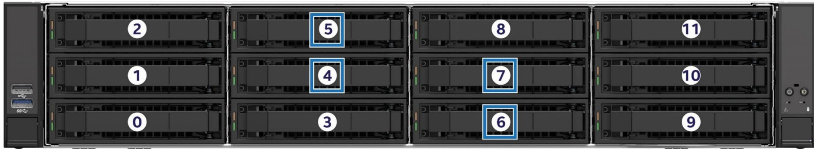
Figure 27. 2U 12 x 3.5" M50FCP2UR312 Front Drive Bay Configuration
