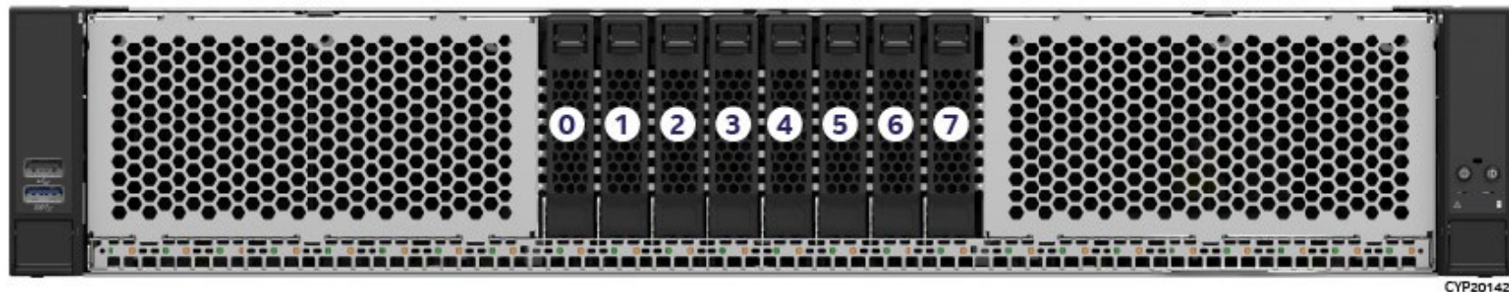
Figure 23. 2U 8 x 2.5" Front Drive Bay Configuration – M50FCP2UR208
