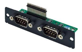
Xpansion Module with 2 x RS232/422/485 (Non-isolation) Support 5V/12V DC Power Output
