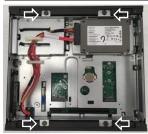
7-1. Loosen M4 screws(x 4) from Mid-Frame.7-2. Loosen M3 screws(x 2) from Rear-Cover.
