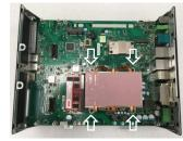
8. Fix CPU heat-sink by M3 screws(x 4, pack 452D80500002) as arrow shown.
