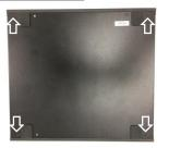
1. Loosen M3 screws(x 4) from Bottom cover as the arrow locations.
