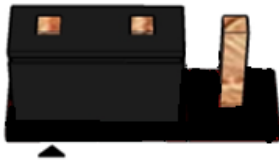
Pins 1&2: jumper position for CMOS Reset
